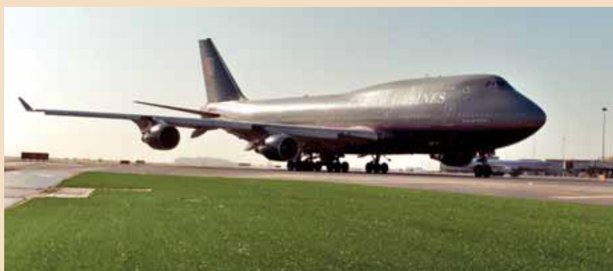
Photo 3. San Francisco International Airport, after installation of artificial turf. In addition to its safety value, the turf provides aesthetic value to arriving passengers.
