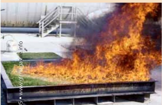
Photo 2. Fire tests found that flames were extinguished quickly, in part because the turf infill snuffs out the oxygen.
